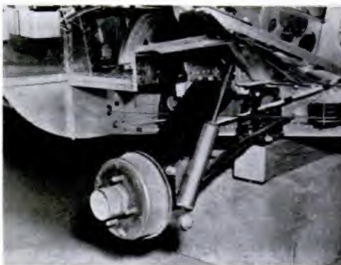
RETRACTABLE WHEELS are extended for takeoff, retracted for flight. A midposition is for road use
